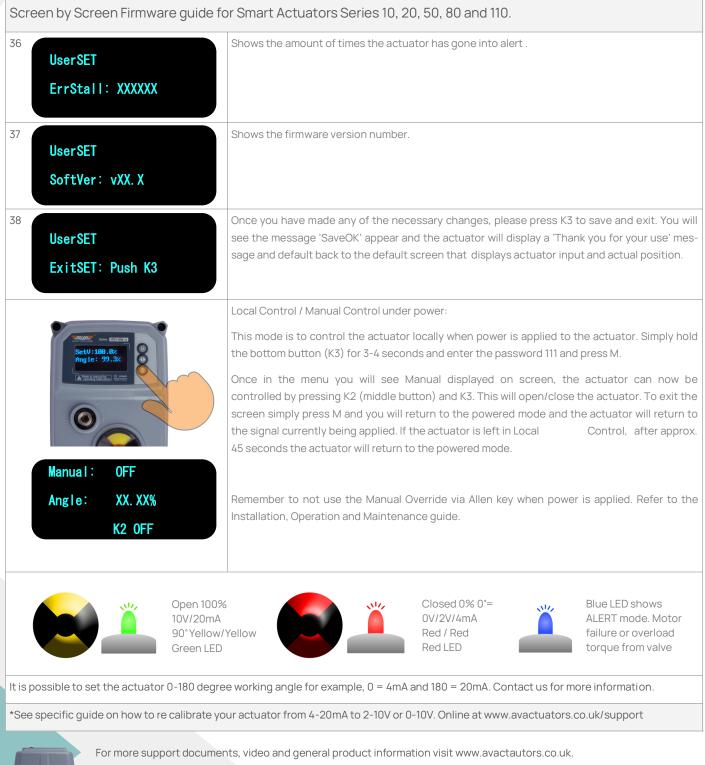
To view other Firmware guides for Modulating actuators and Series 200-400, click on the image of the actuator. As we update our Firmware guides, we will make superseded versions available for download on our website.
